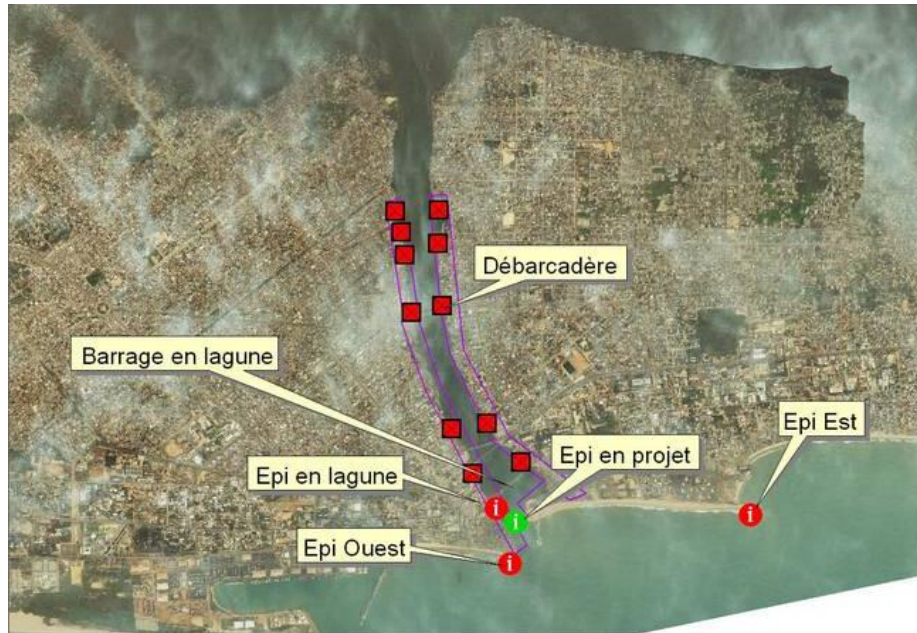
Figure 31 : Physical intervention framework of the project: existing infrastructure, industry to be developed, existing or planned breakwaters, lagoon dam, embarkation/disembarkation and associated infrastructure.
